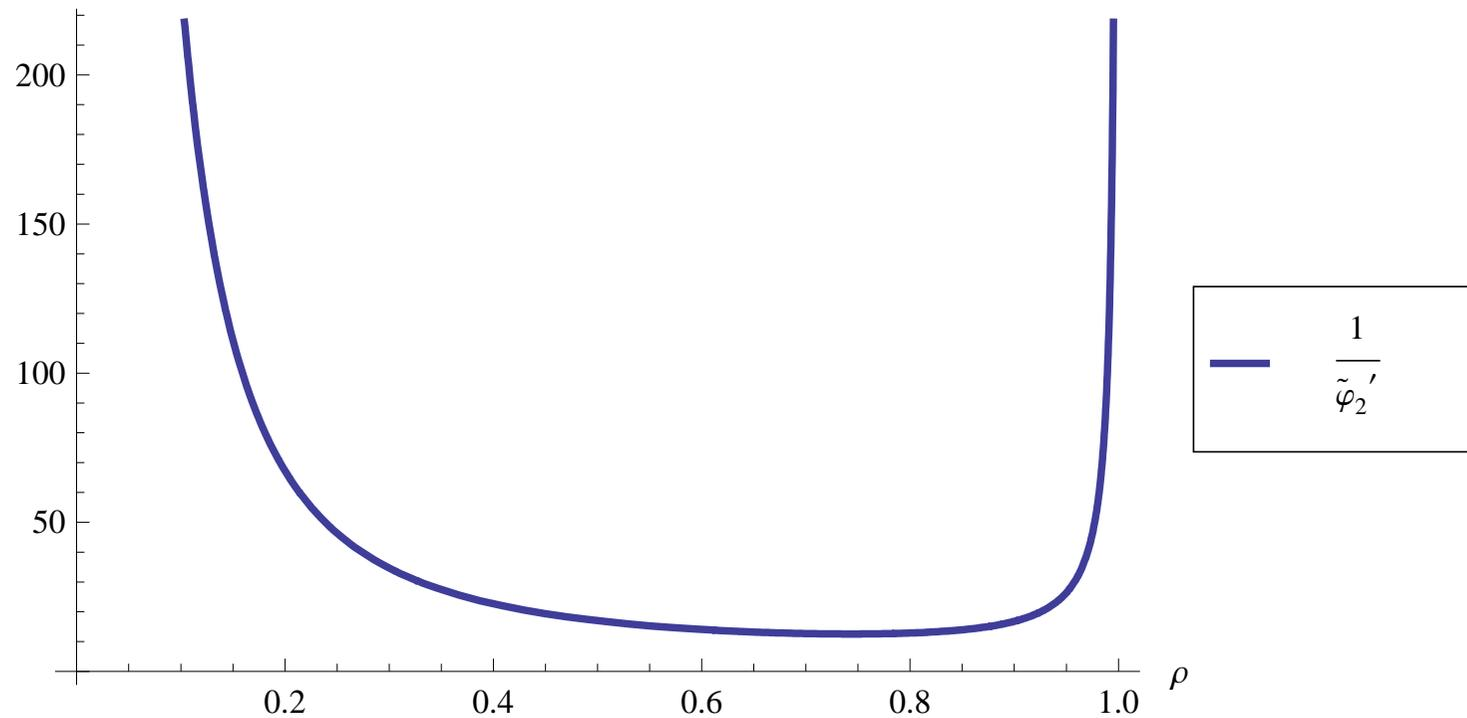
**SHMGQART:** Average system run-through  $\frac{1}{\tilde{\varphi}'_2}$  as a function of the parameter  $\rho$
