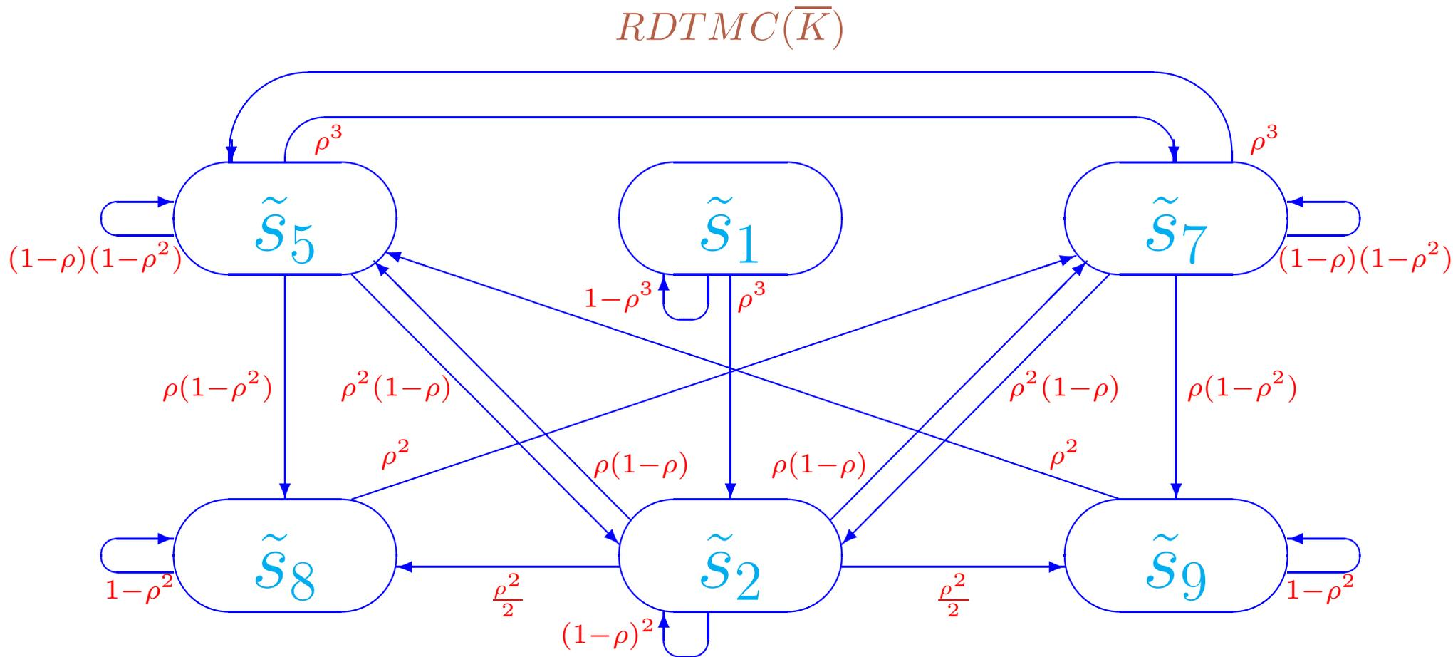
SHMGRDTMC: The reduced DTMC of the generalized shared memory system
